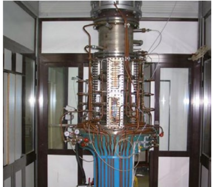
TAO: Optical Test Rig for gas turbine burners and for development of GT view probe
